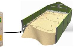
Connect up to 12 crop temperature sensors to a Multi-Sensor Switch and plug in a Minitemp Monitor to create a simple logging system
